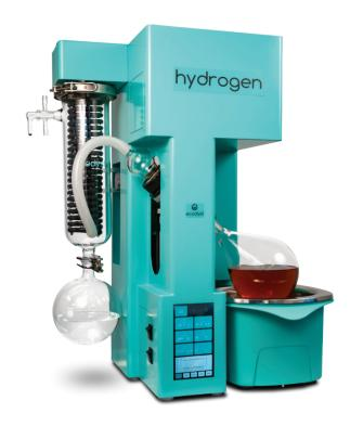
The multipurpose hydrogen from Ecodyst is ecofriendly, energy efficient, reliable, and sustainable. This contemporary rotovap also delivers excellent performance, has a smaller footprint, features an extremely efficient always-available built-in condenser, is more economical to operate and decrease evaporation time, which enables researchers to pay attention to more difficult tasks.
