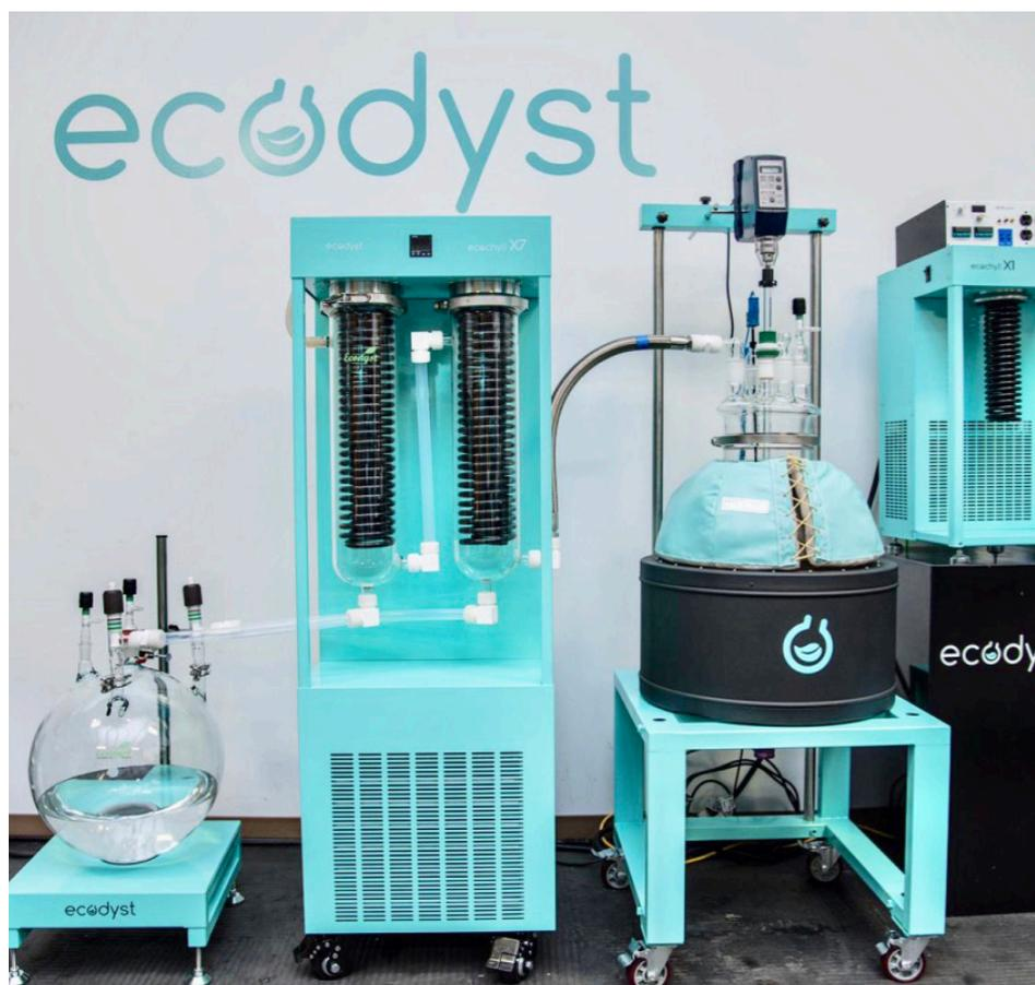
Ecodyst's rotary evaporators incorporate condenser coils that are made from a polymer-coated metal rather than the traditional glass. Combining condenser and chiller into a single unit has proven to be a scalable approach.
